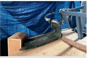
An original piece of copper used as a pattern at the base of the lantern.
